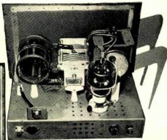
Two views of the two-band final. The chassis and cabinet were constructed of Reynolds "Do-it-Yourself" aluminum.
