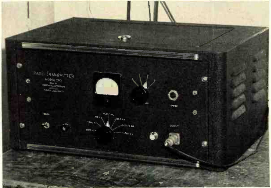
Fig. 5. Transmitter in operation in Cary Hall. One meter and a multi-position switch gives data on all necessary circuits. Transmitter was home constructed.
